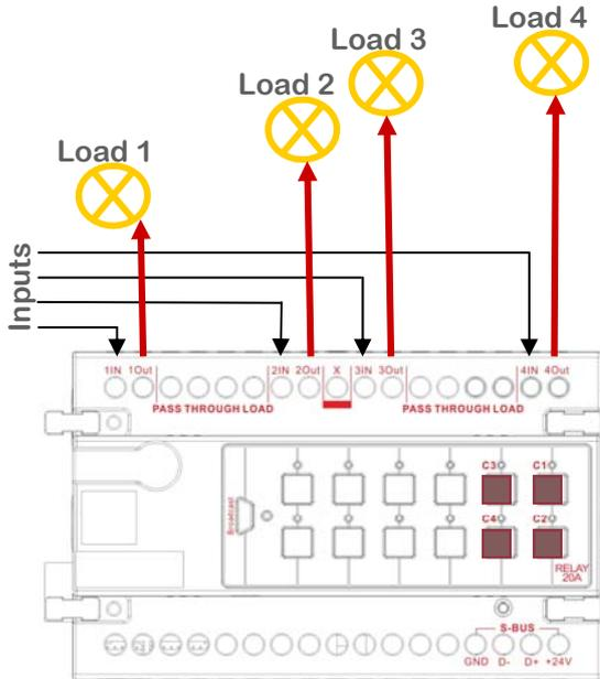
\*Loads Inputs Can be from Different Phases and different Voltage or frequency. Accept ELV: 80-240VAC, and ELC: 1.5-48VDC
